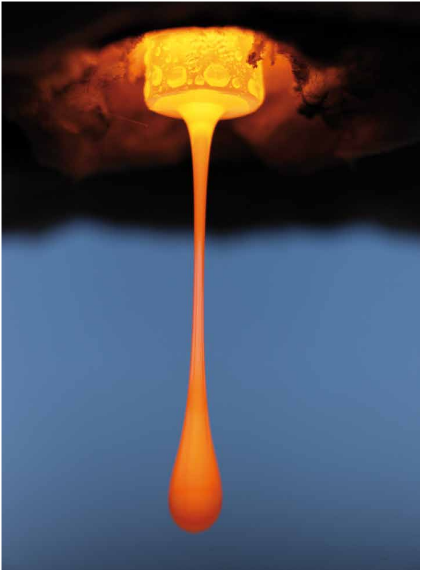
A drop of glass taken out of the induction furnace at Jülich's Central Technology Division, which has a temperature of 1,500 °C. © Jülich Research Centre (FZJ).
